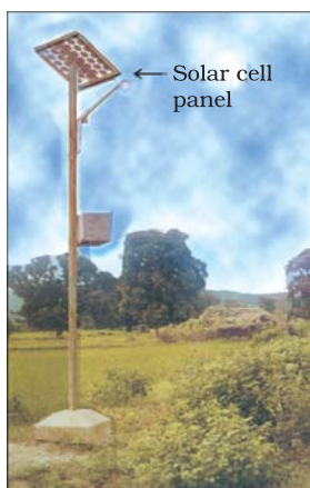
Figure 14.7 A solar cell panel
